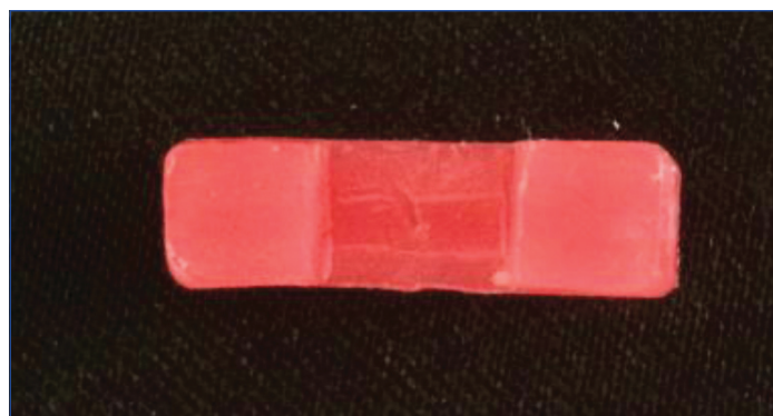
[Table/Fig-1]: Wax pattern with indentation in the centre.
