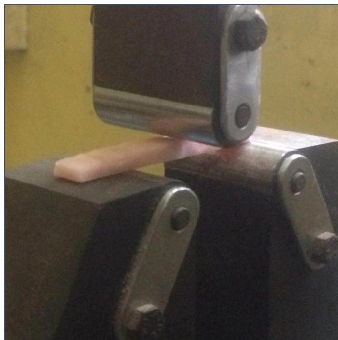
[Table/Fig-4]: Flexural strength tested with universal testing machine.
